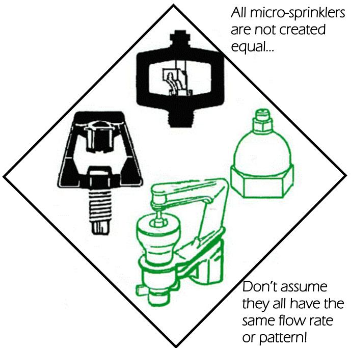
**Micro-Sprinklers** - Another major problem that detracts from a system's emission uniformity is a lack of micro-sprinkler performance. Two of the most common sprinkler problems are:
